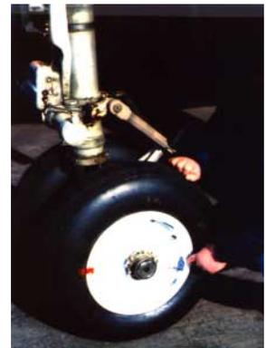
*Loctite® 587 Blue High Performance Silicone does not cause corrosion, protects against de-icing material, and allows for a quick visual check for missing balance weights.*
