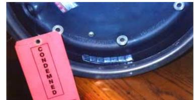
*Corrosion caused by acetoxy-based silicone to the magnesium nose wheels of airplanes, forced an Alaskan-based air carrier to put 16 wheels out of service, costing the company \$90,480 in 1990-96.*
